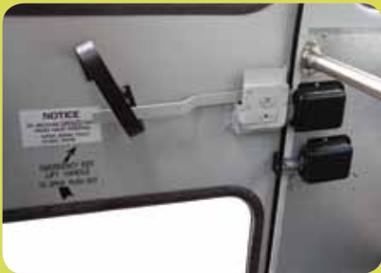
Vandalock - rear door vandal and interlock system
