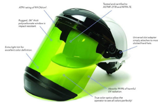
Complete Faceshield Unit with White Six Point Suspension Hard Hat Electric Level II 9.9 cal Arc Flash
