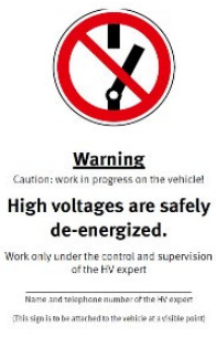
When this sign is posted on the vehicle, it is safely locked-out and tagged-out. You may work on this vehicle under supervision of the SH in charge.
